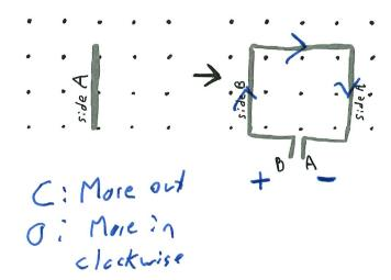
The coil continues its rotation until it is parallel with the field with side B on top.
