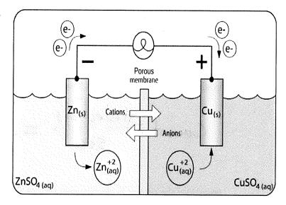
If the anode is connected to the cathode with a wire, electrons from the anode will flow towards the cathode. The electrons at the anode have <u>Electric</u> analogous to gravitational potential energy.
